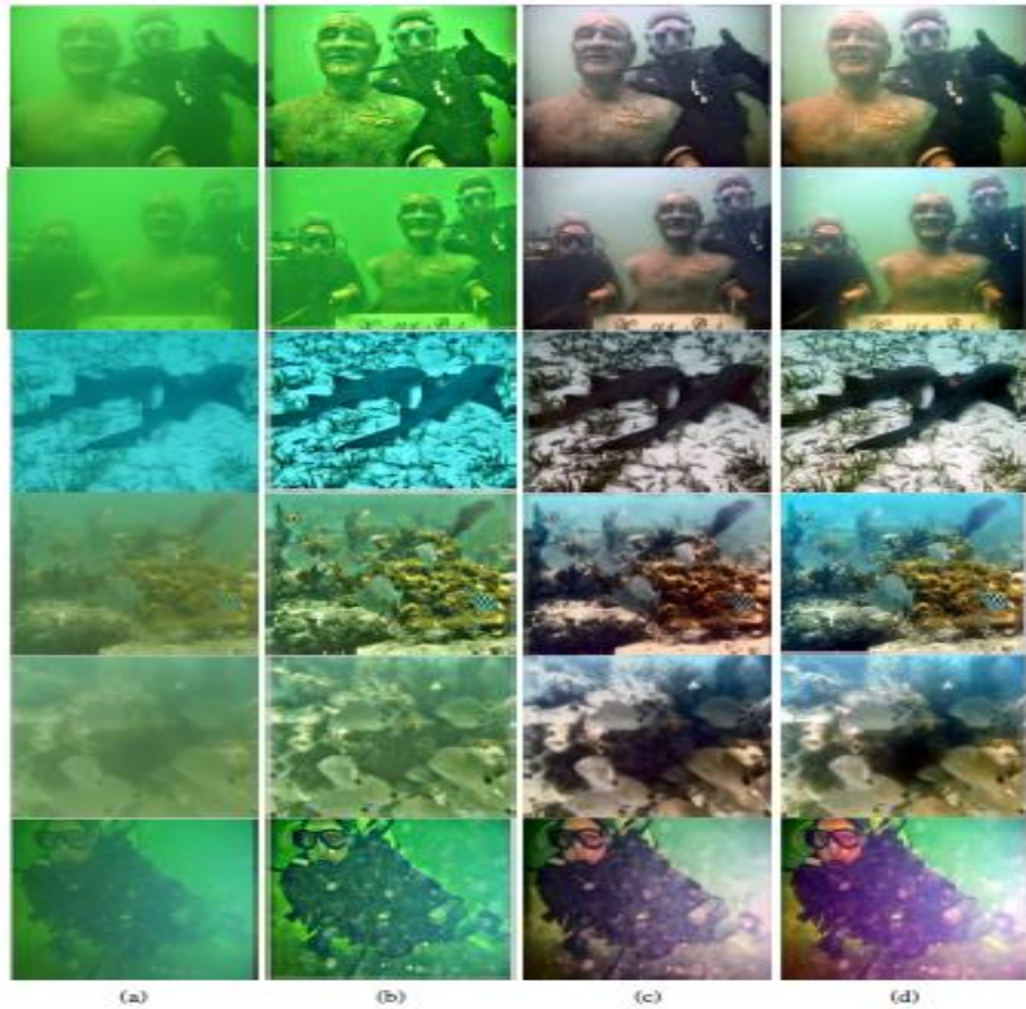
Fig. 2: Results of our fusion method. From left to right-(a) Underwater degraded images, (b) Result from Dark Channel Prior [21], (c) Result from Retinex-based method [22], (d) Proposed method
