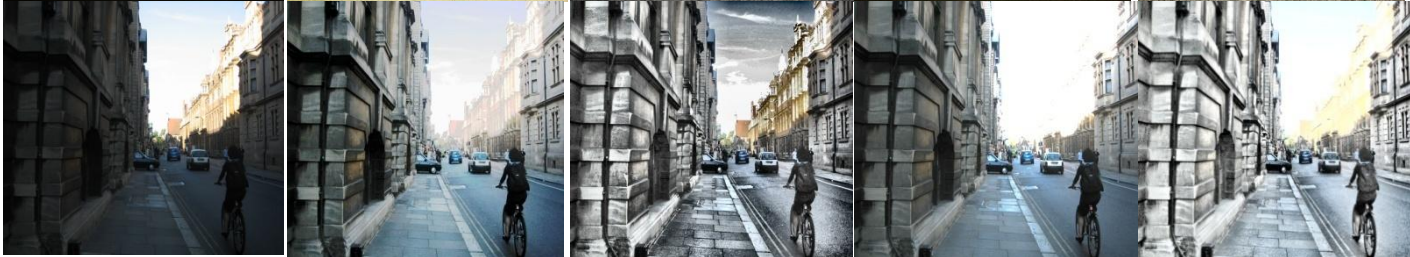
Fig 4.2: (From left to right) Original image, Histogram Equalized Image, CLAHE equalized image, Log-Transformed, Image enhanced in the proposed approach.
